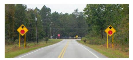
Exhibit 46: Recommended low-cost countermeasures at stop-controlled T-intersection (Source: FHWA)
