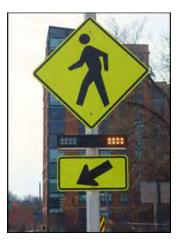
Exhibit 42: An example of a crosswalk high intensity light integrated with an RRFB at night in West Hartford, CT. These lights are only activated when utilized by a pedestrian. Note – The yellow flashers are not activated in this photo to demonstrate the crosswalk light.
